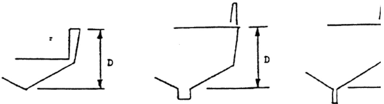
6.4 The measuring of the freeboard is shown in the sketches below.
