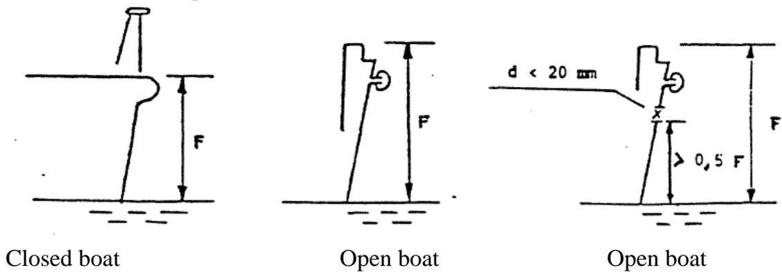
6.5 Example of influence of the location of the cargo and the trim on the calculation of the freeboard amidships compared to the minimum freeboard in accordance with C3.
